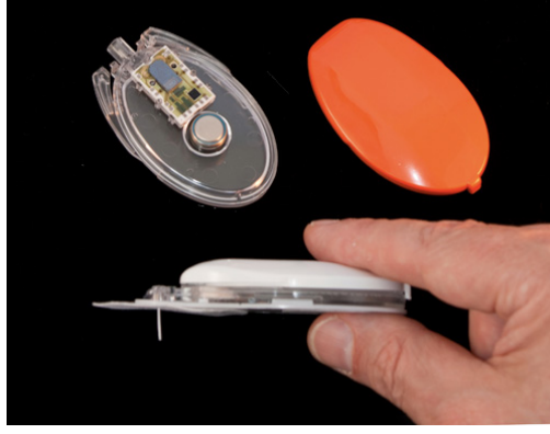
Fig 15 : Subunits of the pump [24]
